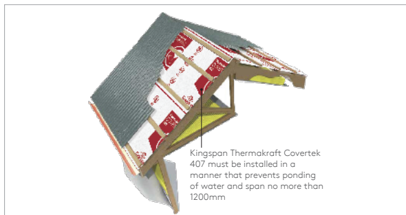
Figure 2. Kingspan Thermakraft Covertex 407 cavity fix.
