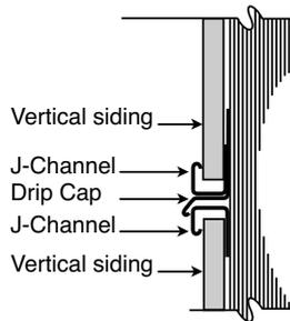
a vertical panel, leave more space at the lower end: allow for 1/3 of the total expansion at the top of a panel and 2/3 of the total expansion at the bottom. For example, if the total expansion equals 3/4" (3/8" + 3/8"), allow 1/4" at the top and 1/2" at the bottom.
