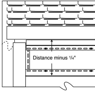
3) Using a square or straight edge, draw a pencil line connecting these points. Then score along line with utility knife. Bend panel back and forth until it snaps.
