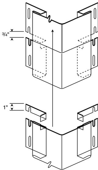
If posts must be spliced for high walls, cut 1" off the nailing flanges and back from the bottom portion of the upper post. Then lap 3/4" of the upper post over the lower post, allowing 1/4" for expansion. This method will provide an obvious joint between the two posts but will allow water to flow over the joint, reducing the chance of water infiltration (shown above).
