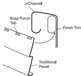
Note: Since you will not nail this last course, it is important that the tabs fit properly in finish trim to provide support while allowing movement for expansion.
