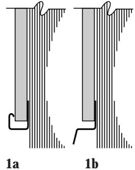
2) Install inverted J-channel along the top of the wall, under the eave. Nail in the center slots every 8" to 10" leaving a 1/4" gap between J-channel and corner posts. Overlap J-channels 3/4" to allow for expansion (see illustration 2b).
